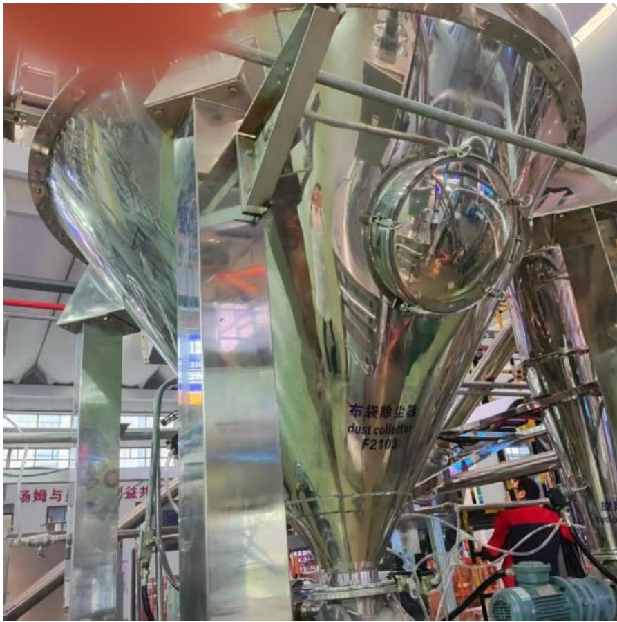
**In the environmental protection section**, dust generated throughout the production process is collected by an air extraction system and treated through environmental protection equipment before being discharged into the atmosphere.
