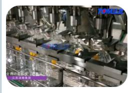
2. Automatically complete operations such as conveying, bottle feeding, self flowing filling, and bottle discharging;
