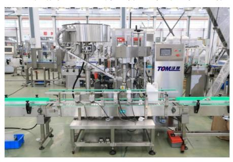
Integrate the inner plug pressing and outer cap screwing into one machine, with one head for pressing the inner plug and one head for screwing the outer cap.
