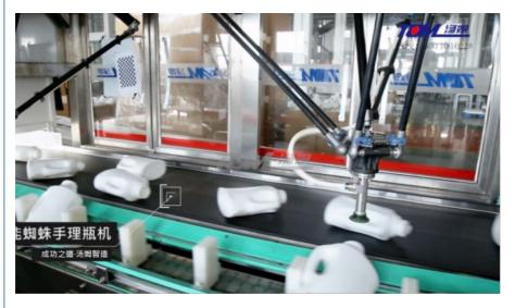
1. It is mainly composed of rack frame, electronic control panel, movable safety door, glass side door, operation panel, side sealing plate and other components. The rack frame is composed of carbon steel welded components and bolted connections.
