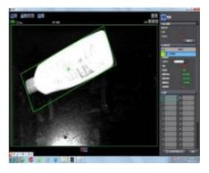
The reverse bottles recognition function can automatically remove the reverse bottles.
