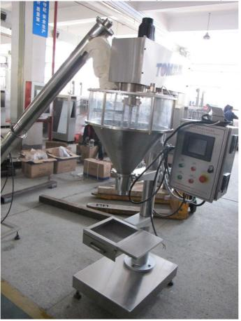
This is powder elevator which is match to semi-auto powder filling machine, when the machine hopper is lack of powder, the elevator will start work, when the machine hopper powder is full, the elevator will stop work.
