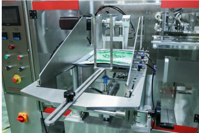
This is the bag outlet conveyor, after filling and sealing, the bag will come out by this conveyor to enter into the next packing station
