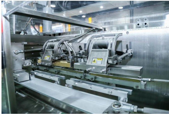
This is the bag feeding part, the people need to put the new empty bags into feeding part manually, usually it can house 200-300pcs of bags
