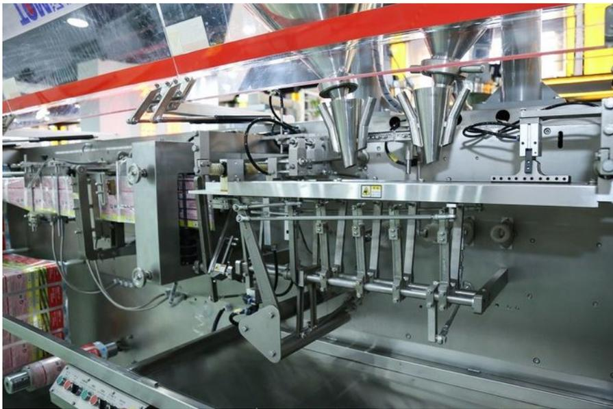
The sachet is formed from film, after forming bag, then filling, after filling then sealing, after sealing then cutting, each movement is accurate, high efficiency.
