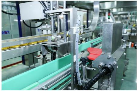
This is the cap sorter, the cap sorter and sorting the caps to capping station one by one automatically, it has linkage function with the cap elevator and capping machine, if the cap sorter bowl is full, the cap elevator will stop feeding cap into sorter, if cap sorter is lacking caps, the elevator will start work again.
