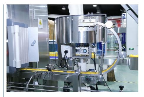
This is the cap transfer station, the capping head will grasp cap here and put cap onto bottle
