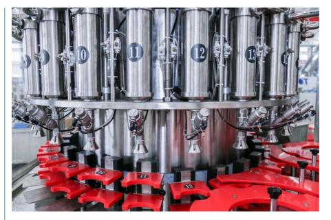
The capping heads suitable for varous kind of caps, and he capping heads are customized according to customer's cap sample, if the cap diameter is different, the capping heads need to change accordingly, but the changeover time is quick.
