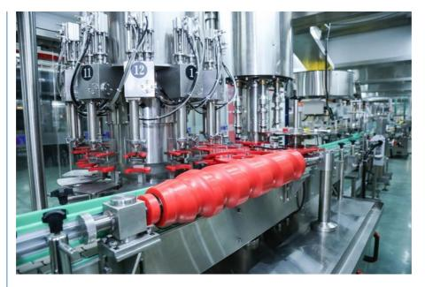
The crooked cap detector and rejector, is the capped bottle is unqualified such as cap is crooked, or cap is missing, this bottle will be rejected automatically
