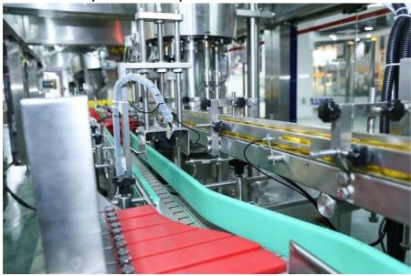
This is the aluminum foild detector and rejector, if the aliminum foil is missing, the bottle will be rejected automatically
