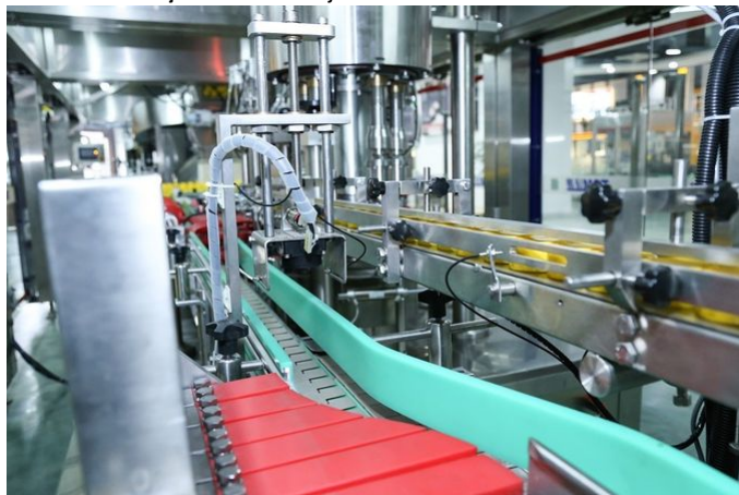
This is the aluminum foil detector and rejector. If the aluminum foil is missing, the bottle will be rejected automatically.
