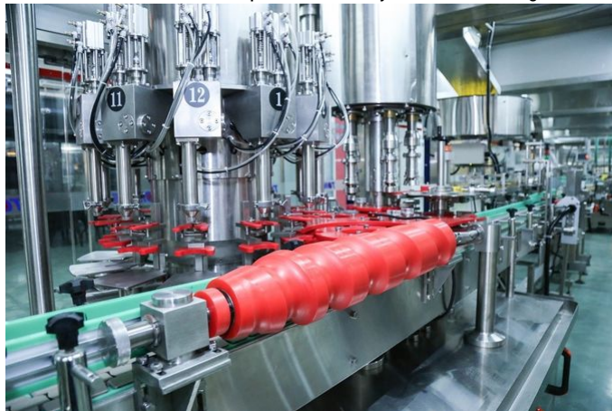
The crooked cap detector and rejector, which detects if a capped bottle is unqualified, such as if the cap is crooked or missing, this bottle will be rejected automatically.
