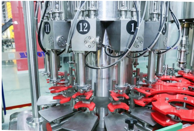
The capping heads suitable for various kinds of caps, and the capping heads are customized according to the customer's cap sample. If the cap diameter is different, the capping heads need to change accordingly, but the changeover time is quick.
