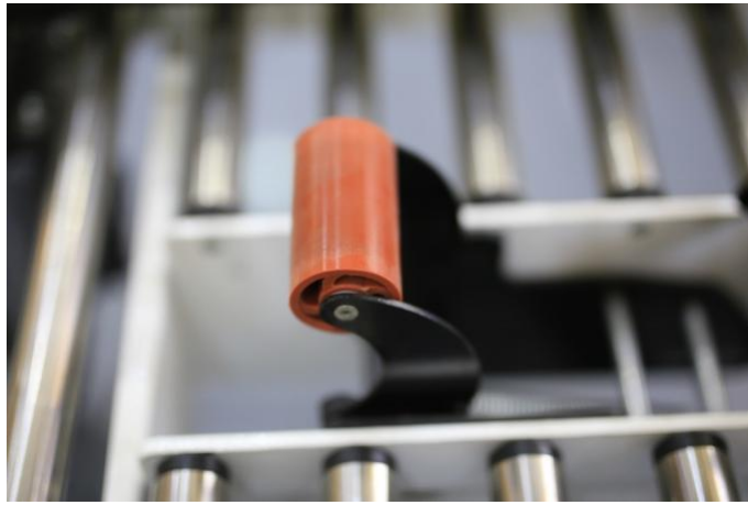
With airtac cylinder control movement, the tape is cut more accurately, avoiding tape waste and saving resources.
