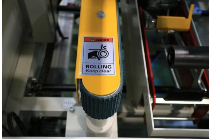
The clamping belt can clamp carton firmly to achieve more good working effects.
