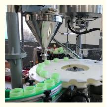
FJ-1BP Fully Automatic PLC Controlled powder packing machine for Bottles
