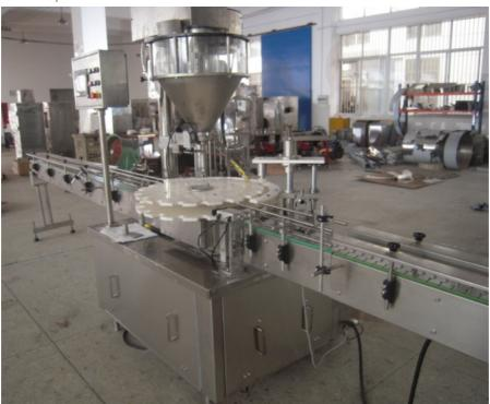
The main components of this machine are all international famous brands. The human-machine interface and microcomputer controller (PLC) adopt the Japanese Panasonic brand. The operation is simple and the operation is reliable. The servo control system adopts Taiwan TECO and has been used by the company for nearly 10 years. Has considerable experience, stable quality, wide application environment and low maintenance rate. The main power inverter adopts the French Schneider brand
