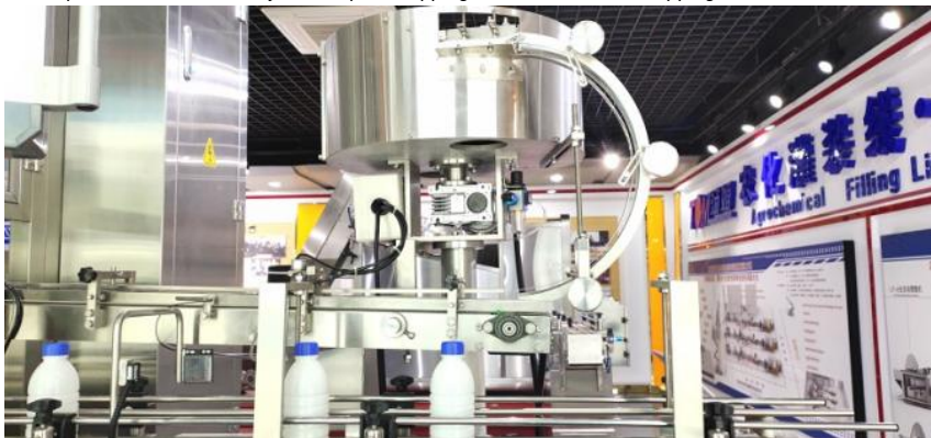
The cap sorter can incessantly feed caps to capping machine, match to capping machine
