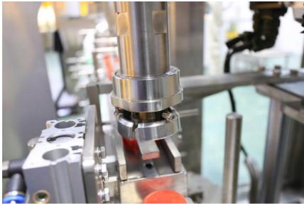
The bottle is clamped firmly by belt during the capping process, and at the same time, it plays the Z-axis direction. The servo motor controls the bottle clamping speed and keeps pace with the capping motor, so that the gripper can precisely match the bottle mouth.
