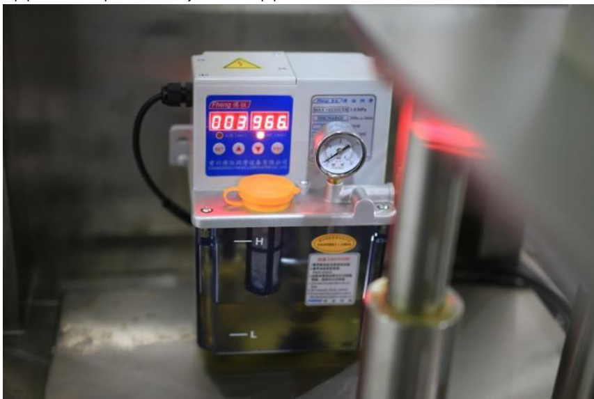
The equipment is equipped with oil pressure distributor and automatic oil pipeline to ensure the lubrication effect of moving parts of the equipment and improve the life cycle of the equipment.
