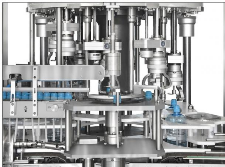
Bottle inlet and outlet star wheel
