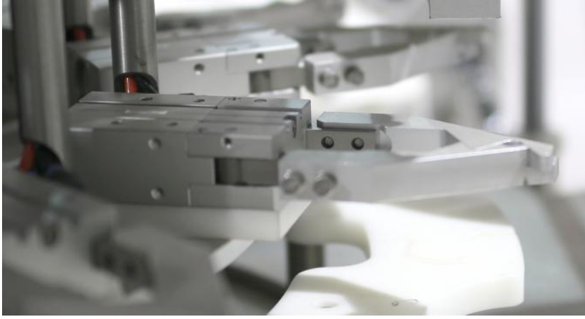
Pump cap/ Trigger cap dip tube centering device
