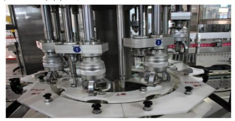
There is ging and disengaging gear motor output station, when plugging bottle or spindle torque overload, machine will clutch automatically, after photoelectric detect dislocation, machine will alarm and automatically stop, protect equipment from damage; Only when people return it to normal position and restart the machine, can work normally.
