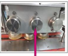
The cap sorter adopts the principle of centrifugal movement to make the cap inside the cap sorter enter the track and do
