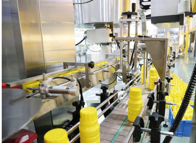
Detection system (if no foil, no cap, have slanting cap will automatic reject)
