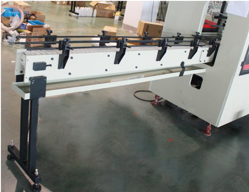
The conveyor and chain plates are all use plastic material
