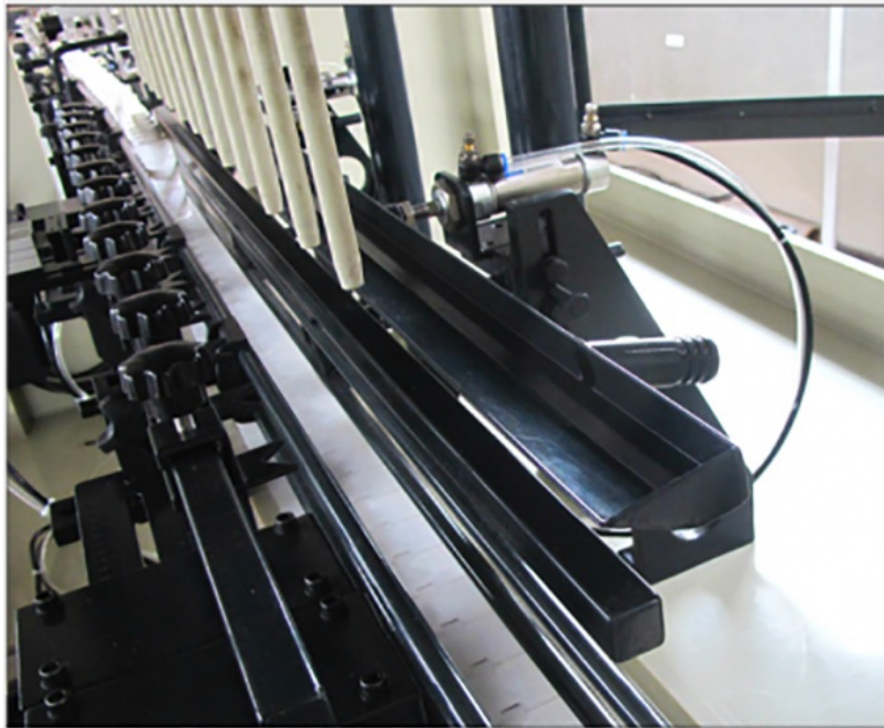
The conveyor and chain plates are all use plastic material
