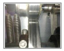
The sealing device wheel frame is all processed by stainless steel castings, which has long service life and strong firmness. The original welded parts are easily deformed and easily broken.
