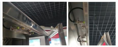
The machine with safety door which can keep operator safe, when open this door, the machine will stop automatically.
