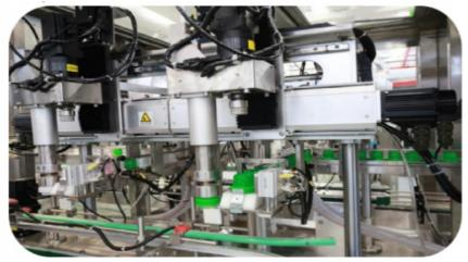
The capping head made with high precision is accurate and reliable. It is made of stainless steel. The surface of the parts is professionally treated. The positions of the three claws are triangular, and wear-resistant dichotomanthes tristaniicarpa are installed inside to prevent direct contact between the metal and the cover and reduce the wear of the cover
